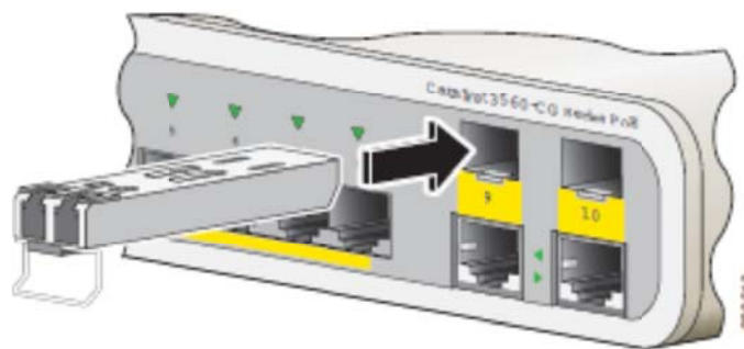
Figure 2-29 Installing an SFP Module
